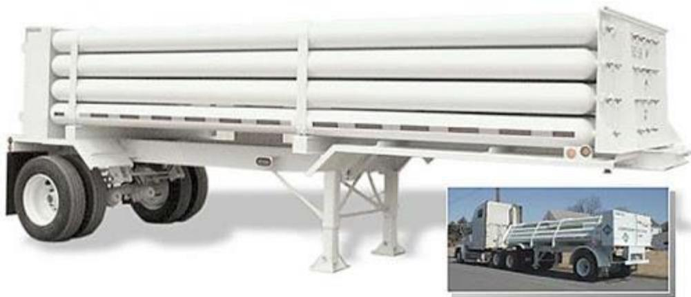
Figure 2: Example hydrogen tanker trailer
